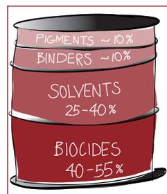
In Sweden anti-fouling paints are regarded as pesticides and must have an approval to be used. In paints applied on vessels over 12 metres only *copper compounds*, "triazine" (Irgarol), "isothiazoline" and zinc pyrithione are accepted as active ingredients. The total biocide content in the most widely used products in Sweden is between 40–55 % by weight.
